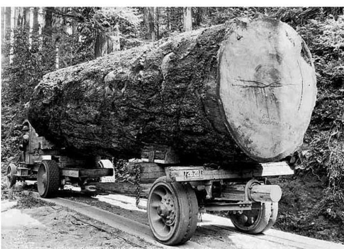
An old single axle Mack, most likely one of the Knutson Nelson rigs on their Miller River job, hauling a massive Douglas Fir log to the mill in Milltown. Note the plank road it is traveling, the hard rubber tires, and the lack of apparent springs. Even at 5 mph it was a rough ride.
